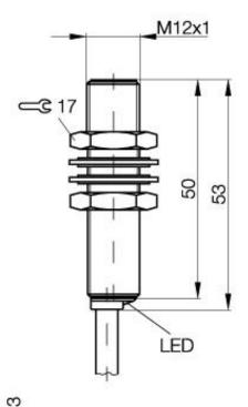
**Inductive Sensors** BES M12MI-POC40B-BV03 M12x1 x 53 normally-closed Sn=4mm shielded
